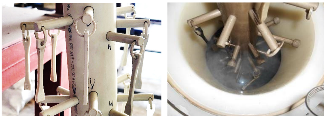
Fig. 2. Equipment used for periodic removal of specimens during testing
