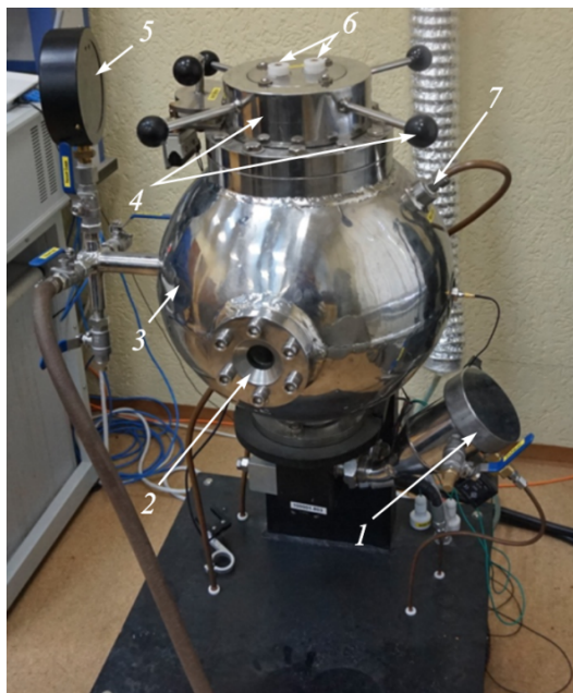
Fig. 1. The installation: 1 – feeding device (dust collector with a volume of 0.6 dm 3 ); 2 – inspection window; 3 – working chamber with an internal volume of 20 liters; 4 – holders and locking mechanism of the 20-liter sphere (working chamber); 5 – manometer; 6 – current conductors (holders of a chemical combustion); 7 – water outlet
