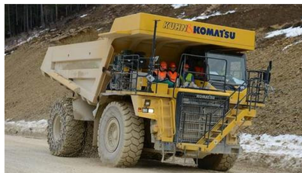
Fig. 3. Trolley truck (battery electric dumper) Komatsu HD 605-7
