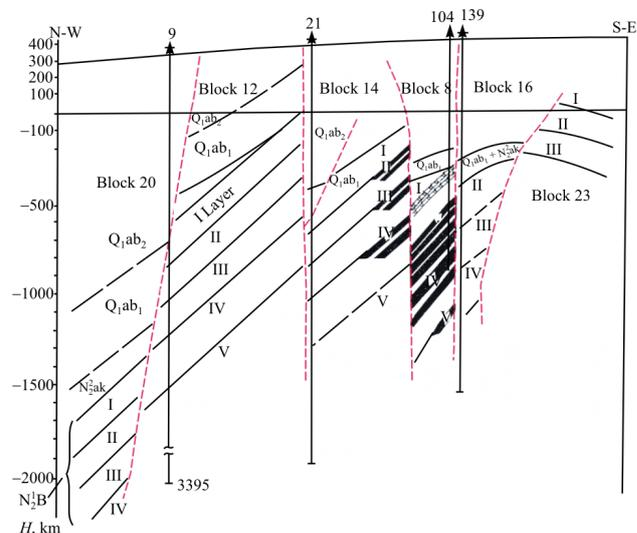
Fig. 5. Kalamaddin fold. Geological profile along the line I-I
