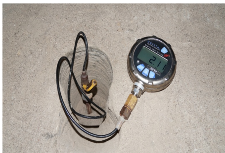
Fig. 3. Measurement of the pressure of free gases on the measuring station using a digital manometer Crystal XP2i
