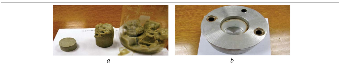
Fig. 2. Behaviour study of montmorillonite clay samples at all-sided and one-sided water saturation: a – from left to right: compression-molded sample before the test; compression-molded sample after the test, placed in a cell and kept in aqueous medium; compression-molded sample after the test, placed in a glass and kept in aqueous medium; b – a cell for compression-molded sample
