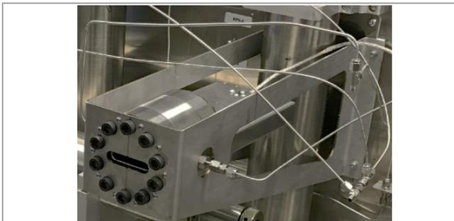
Fig. 3. Cell with a sight glass for checking up on phase behavior of fluids
