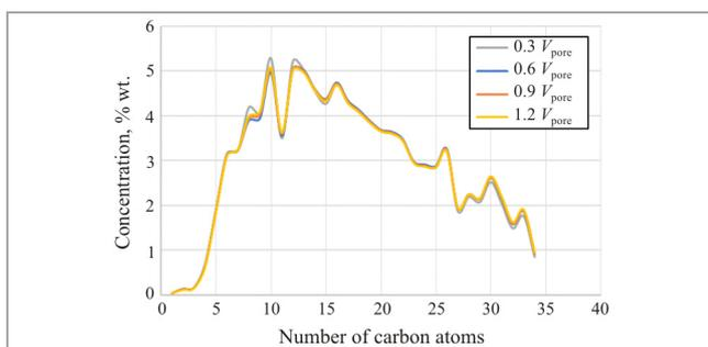
Fig. 8. Compositional analysis of degassed oil samples taken during the experiment performed at 16 MPa using a slim tube
