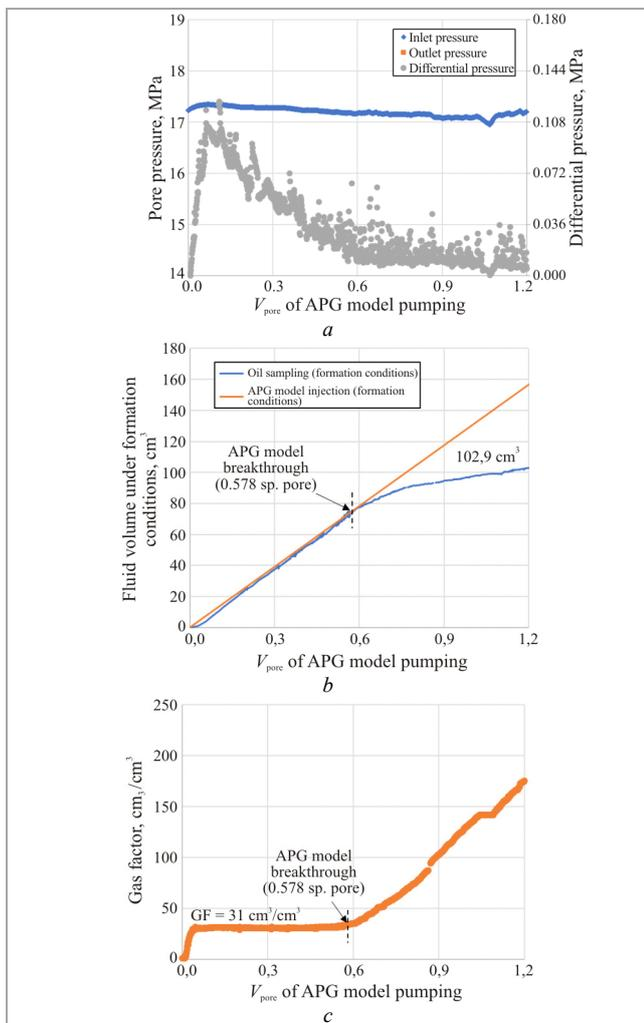
Fig. 5. Standard experiment results: *a* – dynamics of pore and differential pressures during the experiment on determination of the oil displacement factor using slim tubes; *b* – dynamics of oil displacement depending on the volume of the injected APG in slim tube pore volumes; *c* – dynamics of the gas factor depending on the volume of the injected APG in slim tube pore volumes
