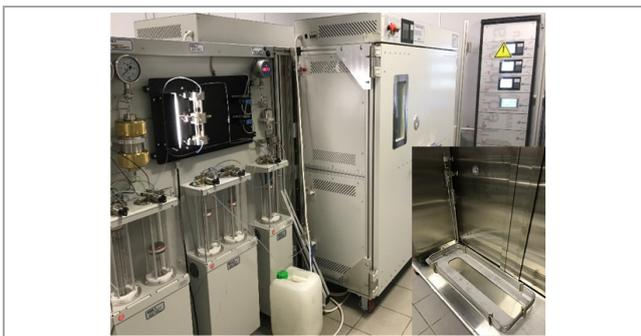
Fig. 2. Three-phase filtration apparatus and slim model in the oven
