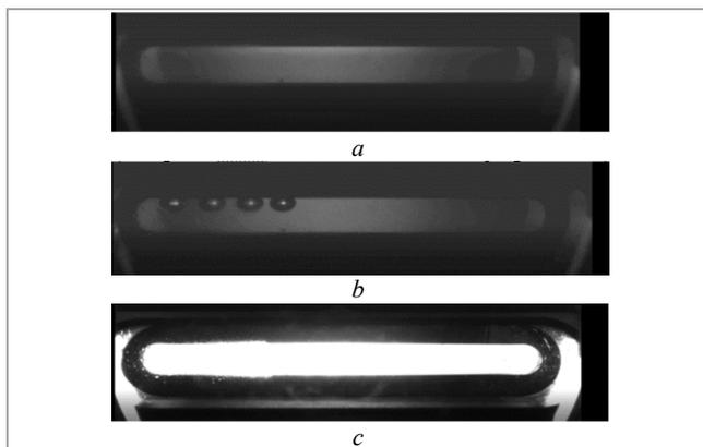
Fig. 9. Results of the visual observation of the phase behavior of fluids as they leave the slim model: *a* – the first experiment stage (set 1, experiment No. 3, 15 MPa, injection:  $0 V_{pore}$ ); *b* – the APG model starts breaking through (set 1, experiment No. 3, 15 MPa, injection:  $0.655 V_{pore}$ ); *c* – the last experiment stage (set 1, experiment No. 3, 15 MPa, injection:  $1-1.2 V_{pore}$ )
