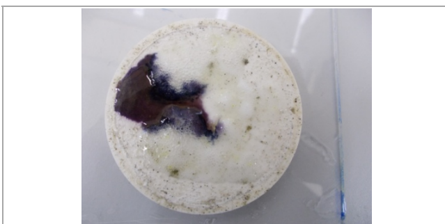
Fig. 4. Discoloring of the iodine solution, indicating the presence of starch in the filter cake
