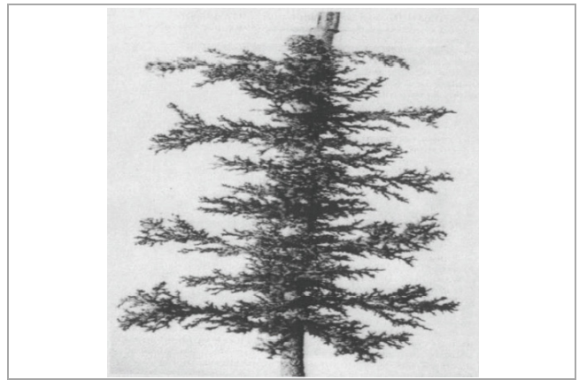
Fig. 2. Channels in the carbonate samples after hydrochloric treatment
