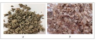
Fig. 1. Sludge when passing through: a – gypsum rock (6,675 m); b – salt formation (7,600 m)
