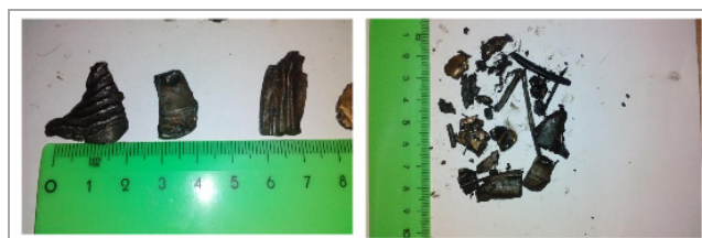
Fig. 4. Photo of metal fragments from the well No. 24 of the Yurubcheno-Tokhomskoye field, raised to the surface during flushing
