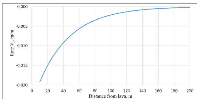
Fig. 5. Graph of convergence rate change "Roof-soil" from the distance to the lava
