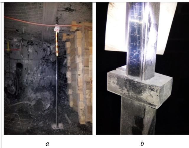
Figure 3. Convergence change device KSH-2 installed in ventilation drift 2-7: a – general view of the convergence meter in the mine workings; b – measuring scale of the convergometer
