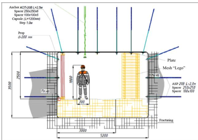
Fig. 2. Scheme of reinforcement of the ventilation drift 2-7 with strengthened wooden support, wooden props and anchors
