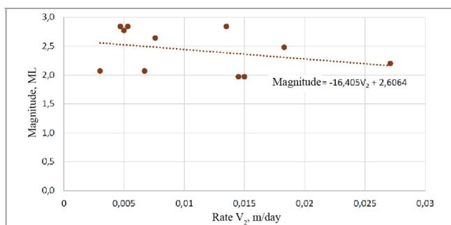
Fig. 6. Graph of dependence of seismic event magnitude on the convergence rate  $V_2$  of the roof and soil of ventilation drift 2-7
