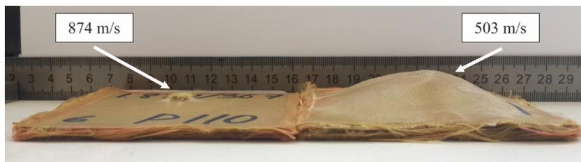
Fig. 2. KV110P/LDPE panels impacted at different velocities
