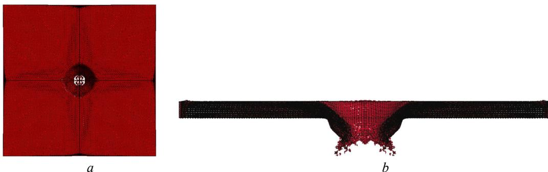
Fig. 9. An example of a numerical simulation of KV110P/LDPE laminate impacted at a velocity of 550 m/s: *a* – front side; *b* –sectional view
