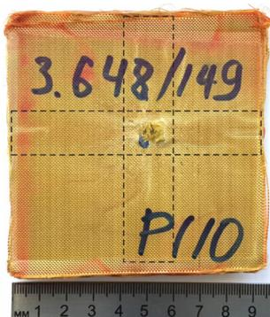
Fig. 3. Buckling area (limited by dashed lines) on impacted side of KV110P/LDPE panel
