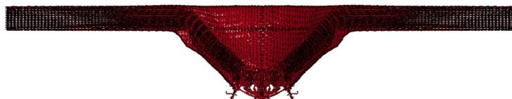
Fig. 10. Sectional view of KV110P/LDPE laminate impacted at a velocity of 500 m/s
