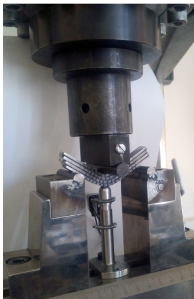
Fig. 7. Multilayer specimen for three-point bending tests with reference lines applied to record interlayer shear
