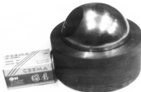
Fig. 9. Shut-off valves with sealing surfaces hardened by wear-resistant electron-beam surfacing of powder alloys in vacuum
