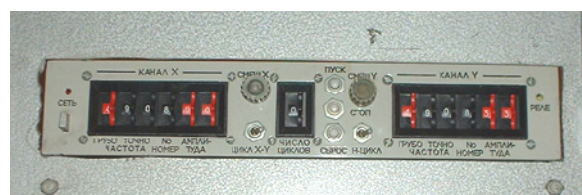
Fig. 2. The panel of the developed electronic beam control software device for the process of welding and hardening in vacuum
