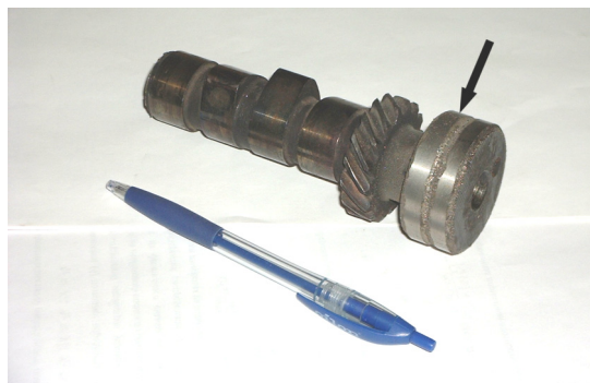
Fig. 8. The camshaft of the internal combustion engine after repair using powder electron-beam welding in vacuum
